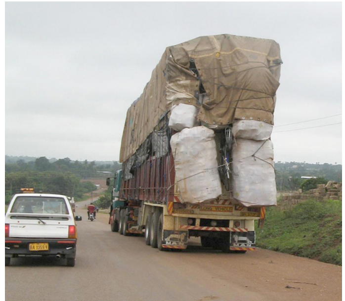
Overload is a severe problem in a country with few resources. The roads are still under destruction in spite of laws against overloading.
